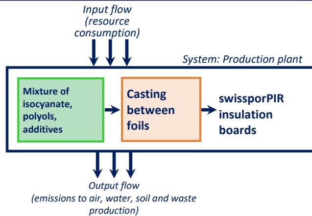
Simplified representation of the processes in the manufacturing phase (phases A1 -> A3)
