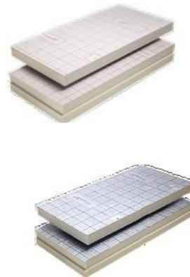
These are rigid boards installed on roofs (flat or pitched) or floors (under subfloor/screed). The thermal conductivity of the insulation boards is between 0.020 W/(m.K) and 0.027 W/(m.K).
